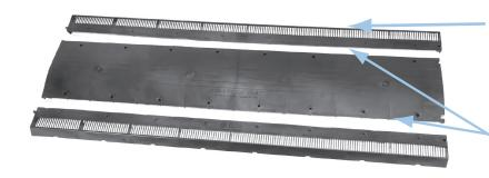
For 10" use, cut groove on underside of vent. Detach and reset one baffle by inserting baffle nail hole into body nail hole.
